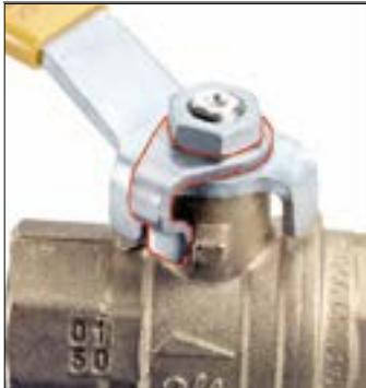
Memory Stop allows to control flow passing through the valve by curbing ball movement from fully closed to a preset position. Installing a memory stop on a standard **RuB** valve is very easy and can be done even while valve is being used.
