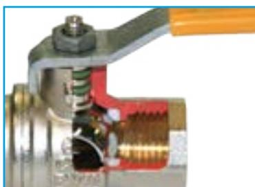
We have also reversed handle: in this version the handle is parallel to the pipe when the valve is closed and perpendicular when the valve is open. This option is available only in the small size for valves up to 1/2" (or 3/4" for reduced bore)
